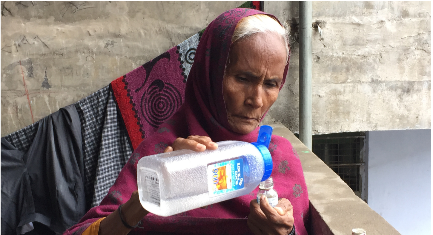
Field test participant Asma Patham performs a H_2S test on the steps of her apartment complex in the Khodiyarnagar neighborhood of Ahmedabad. She used to purify her water using a reverse osmosis (RO) filter, but no longer does because she believes that the tap water is clean. Both her test samples yielded positive results. Credit: Jonars Spielberg
