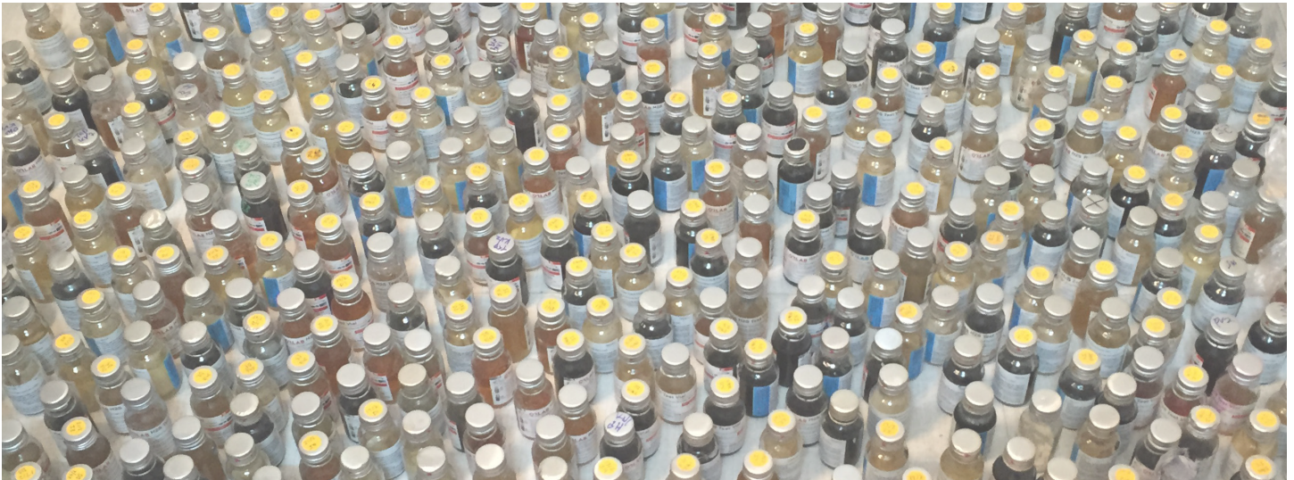
Results from several single parameter, hydrogen-sulfide ( H_2S ) water tests taken from samples in Ahmedabad, India. Credit: Jonars Spielberg
