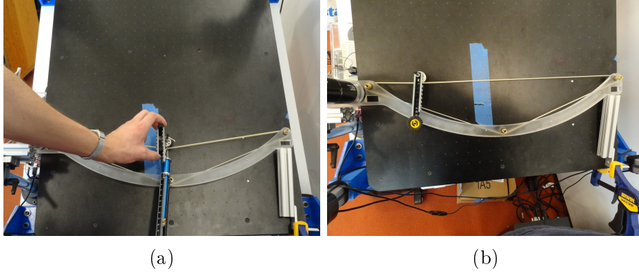
Figure 3-1: The experimental setup used to validate our model. A rubber band stretched taught between two pulleys serves as our soft membrane. Force is measured at a number of deformation points of the cable, stretching the cable down to each such point. The force was characterized via two types of measurement: (a) the vertical component of the force was measured using a linearly-constrained strain gauge apparatus with a roller wheel at the interface to the band, and (b) the angle of the force at every point was measured using a swiveling apparatus which was free to rotate to a minimal energy orientation, also with a rolling interface. For this second device, the measurement was the angle made by the device when the roller was made to settle at \vec{p} .
