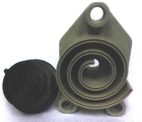
Figure 11 – A scroll pump consists of a fixed and rotating set of involutes. PTFE seals at the face of each scroll help seal the pump and reduce leakage
