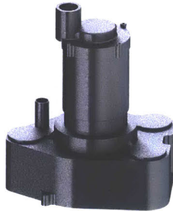
Figure 10 – A CAD rendering of the MOXIE scroll pump design
