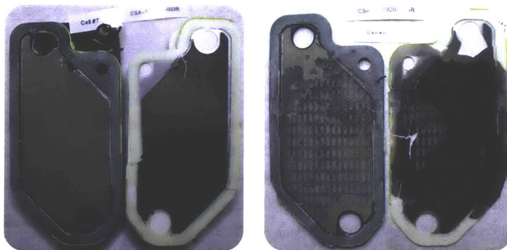
Figure 19 – CSA 003R SOXE cell cathode without signs of coking (left) and with significant coking (right)
