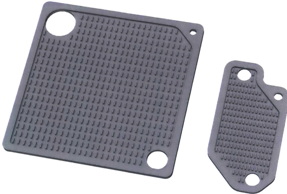
Figure 92 – A notional crewed mission scale SOXE interconnect with an active area of 100 \text{ cm}^2 (left) compared to a MOXIE cell with an active area of 22.74 \text{ cm}^2 (right)
