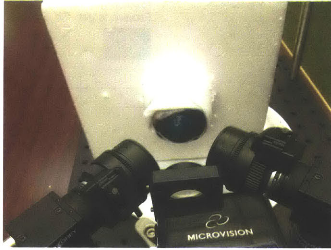
Figure 4-6: Experimental setup of one and two lens models for data capture on bovine, porcine and rabbit eyes ex vivo .
