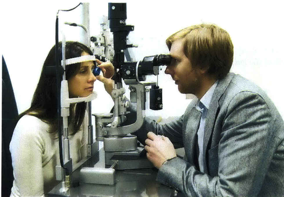
Figure 1-2: A conventional benchtop slit lamp. The optics of the device do not make it large - it is ergonomic to have a chin rest and to have the device mounted on a stable platform like a table. In this image the clinician is using an additional handheld lens to examine the retina. (Photo from [3].)
