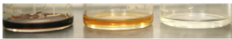
Figure D-6: [emim][Tf 2 N] before and after the long-duration electrolysis test. The clear liquid is [emim][Tf 2 N] before it has been electrolyzed. The orange liquid is the result of the 5 V test. The darkest liquid is the result of the 15 V test.
