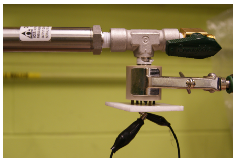
Figure D-3: Pressure vessel electrolysis cell with two 0.5 mm Pt electrodes. Power supplied by Keithley 2410 SourceMeter.
