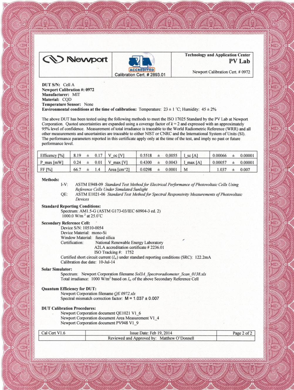
Figure G.2 Certified performance for a high fill factor device. This device was certified after 131 days of air storage and showed the highest FF of 66.7% in QD solar cells as of 2014. The nominal total device area for this device is 5.44 \text{ mm}^2 defined by the overlap of the anode and cathode. For the certification, a 3 \text{ mm}^2 mask was attached to the device to define the device area.
