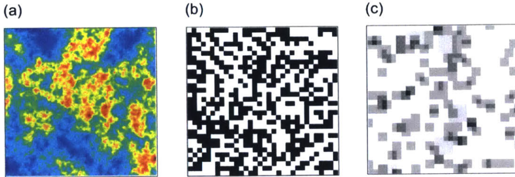
Figure 1.3: Examples of random fields from the a lognormal, b checkerboard, and c random inclusion models considered in this thesis.
