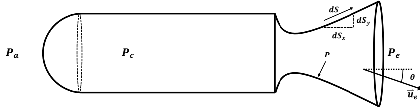
Figure 4-5: Stress considerations for a thermo-chemical rocket. The static pressure in the chamber of the rocket, P_c , is high and typically owes to exothermic reactions between an oxidizer and a fuel. High pressure gas from this chamber is convectively accelerated through a nozzle where it exits with a pressure P_e that may differ from the ambient P_a . The integral of the pressures acting on the solid surfaces of the rocket plus the momentum exchange embodied by the exhaust gas defines the total thrust powering the vehicle.
