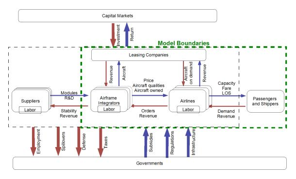
Figure 5: Commercial Aviation Enterprise Structure and Model Boundaries
