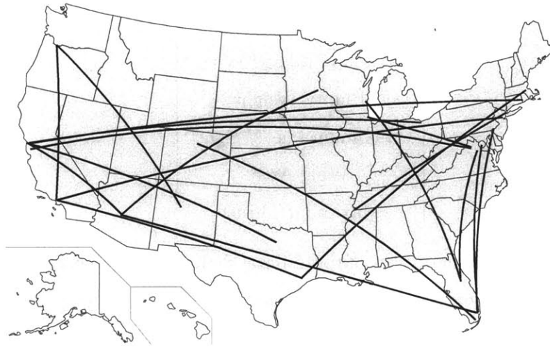
Figure 5-3: Illustrated here are the 20 representative flight trajectories flown by the Boeing 737-800W in the TASOpt-AEDT uncertainty quantification study.
