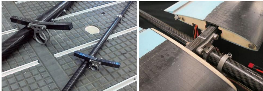
Figure 15: two sizes of wing joiners (left) with wings (right)
