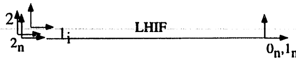
Figure 6-20: A schematic showing the coordinate frame locations on LHIF after 1 st assembly operation
